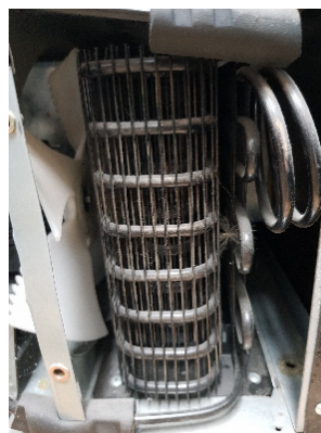
Figure 9: Lightly soiled condenser.
