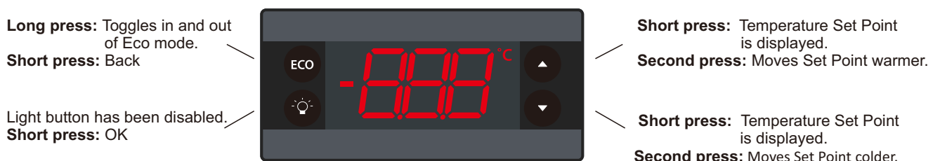
Figure 5: Fascia of the control panel
