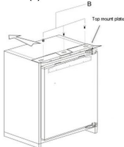
NOTE: Do not over tighten the screws when installing the "top mount bracket", so the bracket can be aligned left or right, when in the cabinet.
