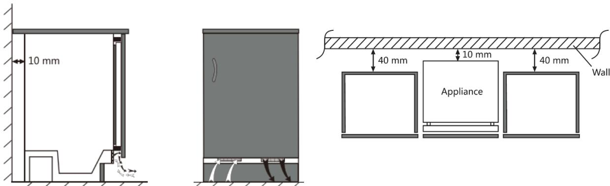
NOTE: This fridge/freezer vents through the front grills. Care must be taken to not block/obstruct these air channels. Allow for a minimum of 140cm<sup>2</sup> of air flow, calculate using Width x Height (20cmW x 5cmH = 100 cm<sup>2</sup>). Most times the door is forward more than fridge, with skirt board behind, leaving a gap for venting that is effectively 'hidden'.
