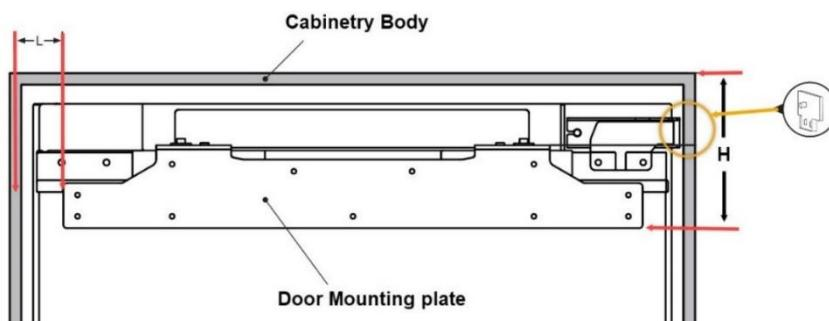
NOTE: Depending on cabinetry layout, L, will be either flush with end of vertical wall of cabinet body, OR half distance of cabinet wall thickness, if sharing cabinet carcass wall with another cabinet door. Ensure you allow for a standard 2-2.5mm gap between cabinetry panels/doors if sharing carcass wall.
