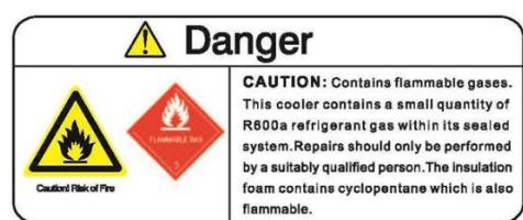
It is hazardous for anyone other than an authorised service person to service this appliance. In Queensland, the authorised service person **MUST** hold a Gas Work Authorisation for hydrocarbon refrigerants to carry out servicing or repairs which involve the removal of covers and the opening of refrigeration piping system.
